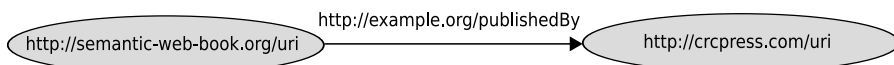
FIGURE 2.1: A simple RDF graph describing the relationship between this book and the publisher, CRC Press
